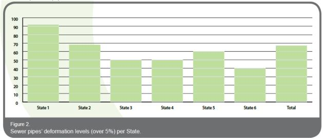
**Condition grading study in six US States:** A study survey was carried out in 2002 to investigate levels of deformation in plastic pipe networks installed since 1987 in six American states. The results were significantly alarming and showed what could be the real scale of the problem in these states as 69% of the pipes inspected had deflections exceeding 5%.
