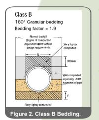
**Concrete pipes** are **rigid** pipeline systems that do not deform, utilising their **inherent strength to withstand loads** and stresses. They receive additional structural support from the soil underneath and around the pipe. Typically, 60 to 100% of the design atomath of a pipeline in built into the pipe ited.
