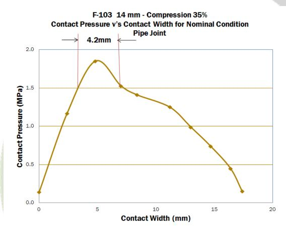
Allowing for up to 45% stress relaxation of the seal over time, this joint design together with the concrete pipe surrounding it will remain watertight in excess of 120 years.
