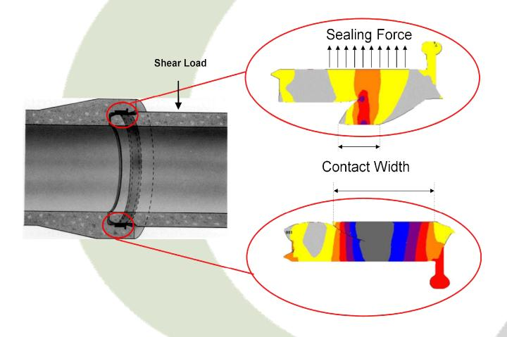
The integrated seal pipe joints currently used in the majority of pipe joints not only achieve the 0.15 MPa mean sealing pressure requirement but actually achieve 0.49 MPa exceeding the minimum requirement by 325% !
